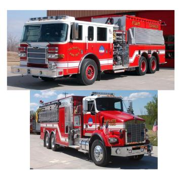
A tender is the water hauling backbone of SPFPD in rural areas. Each tender is equipped with a pump, a large water tank, a complement of ladders and a portable folding tank. The portable tank is a small, temporary reservoir from which an engine can draft water and pump through hoses.
