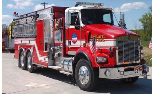
A tender is the water hauling backbone of SPFPD in rural areas. Each tender is equipped with a pump, a large water tank, a complement of ladders and a portable folding tank. The portable tank is a small, temporary reservoir from which an engine can draft water and pump through hoses.
