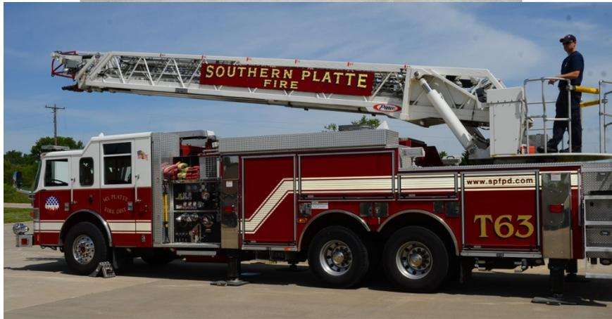
An engine is the day-to-day workhorse of SPFPD. Each one is equipped with a pump, a water tank, a complement of ladders, and thousands of feet of hose.
